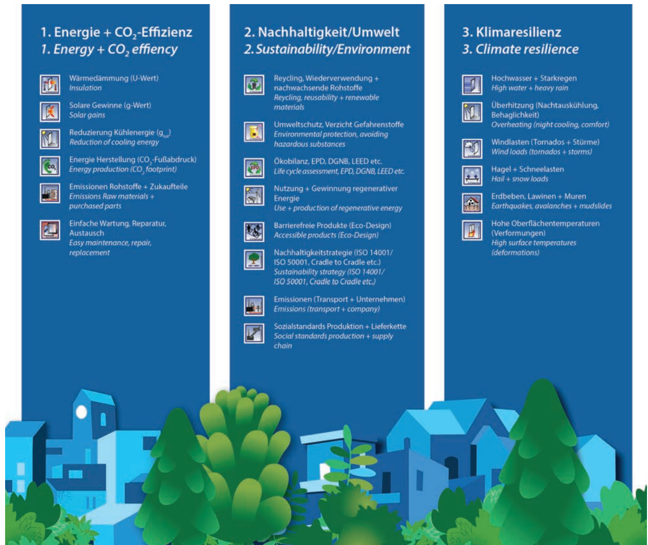
Fig. 25 Aspects for climate-proof building elements
