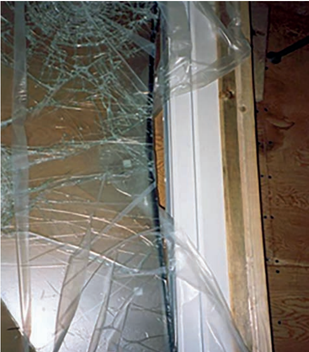
Fig. 14 Testing of hurricane-proof building elements at ift Rosenheim according to [22]
